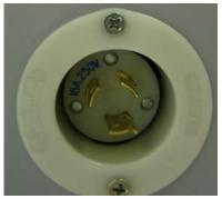
Connect the power cord to the power entry module on the side of the aspirator and to the power source. Note: Be sure your power is labeled "Hospital Grade" and that power required matches power supplied.
