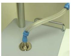
Connect the "PUMP" end of the HEPA filter to the vacuum port on the top of your aspirator.
