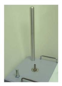
Attach canister support rod into threaded hole on the upper right corner of device.
