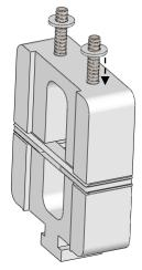
7. Screw the two nuts (part L) onto the bolts in order to secure the cutting jig together. Firmly tighten by hand.
