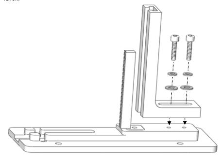
2. Slide the sliding post (part B) into the main base.
