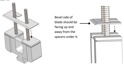
5. Slide the cutting jig (front component; part E) through the bolts.
