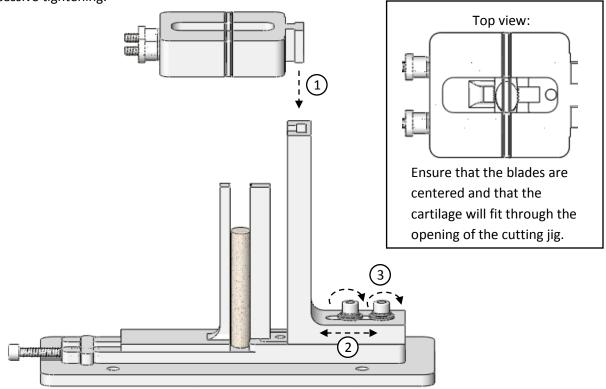
4. With a steady downward force, push the cutting jig through the cartilage.
