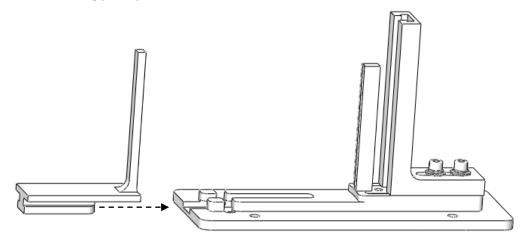
3. Partially screw the bolt (part I) into the clamping bar (part C); several rotations of the bolt is sufficient. Then, place the clamping bar into the inset of the main base.
