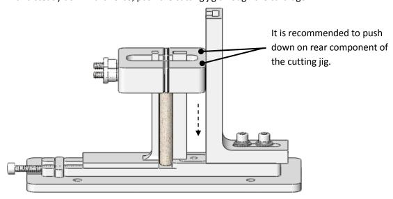
5. Once the blade has reached the bottom and the cartilage is cut, loosen the horizontal bolt that is attached to the clamping bar and loosen the bolts going through the guide. Then, remove the cutting jig and cartilage.
