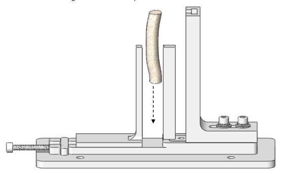
2. Tighten the horizontal bolt that goes through the clamping bar in order to compress the cartilage between the posts. Compress the cartilage to flatten any curvature and to secure it tightly in place.
