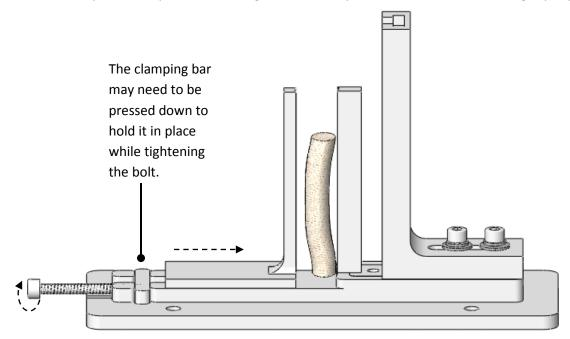
3. Slide the cutting jig through the guide until it rests on top of the cartilage. With the bolts of the guide loosened, position the guide so the blades of the cutting jig are between the posts and at the center of the cartilage. Once the cutting jig is properly positioned, secure the guide by tightening the two bolts. The bolts may be tightened using the supplied wrench, but be careful not to damage the device by excessive tightening.
