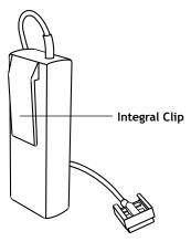
Battery Pack attaches to belt using integral clip FIGURE 2-5
