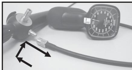
Fig 9. Connection mechanism of leak tester
