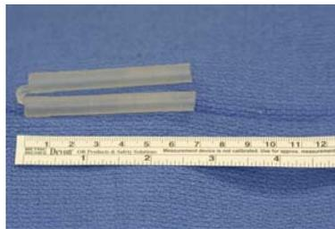
Figs. 12. & 13. Tubes shortened to match probe-determined length of nasal passage.
