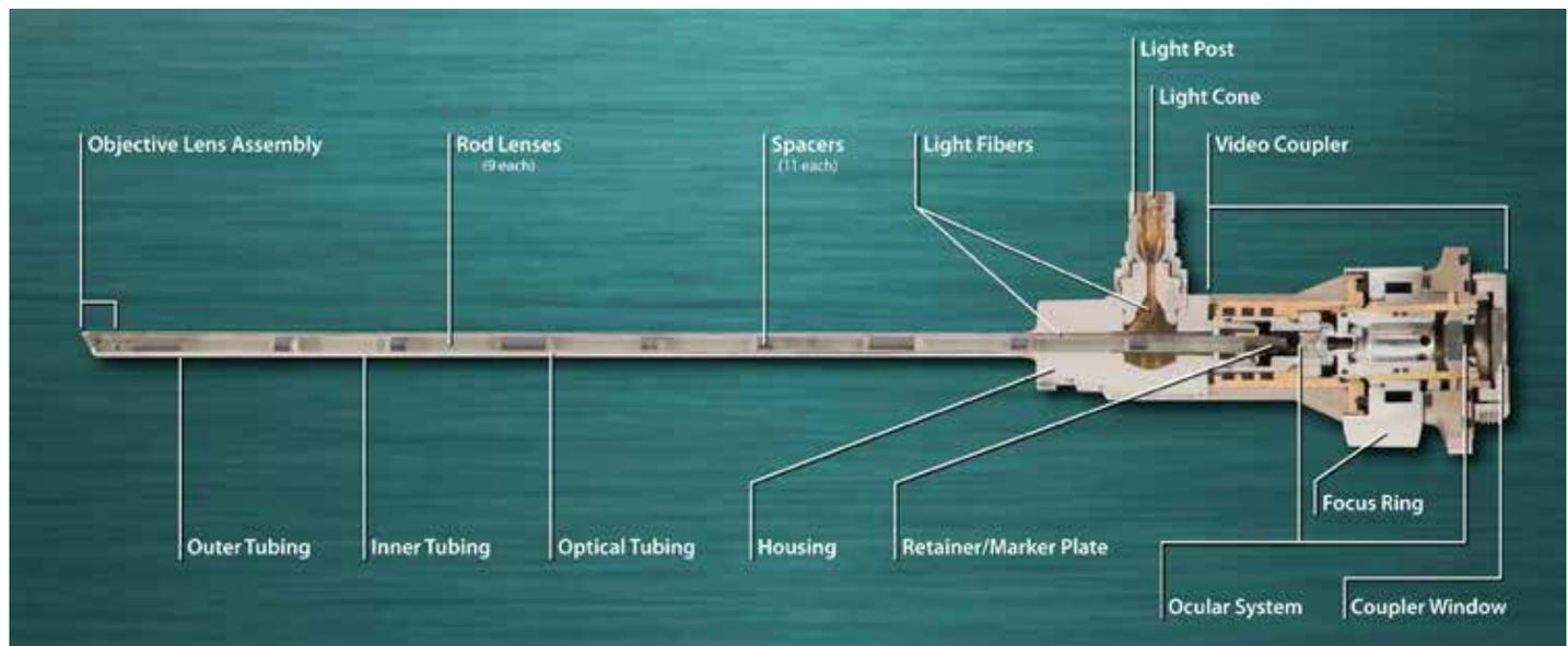
**Eyepiece** – At the proximal end of the scope. Can be used to view through the scope or to attach a Camera Coupler.
